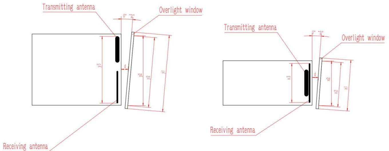
The effective aperture of the optical window  $y_2$  - the outer diameter of the optical window  $y_1 > 2\text{mm}$
