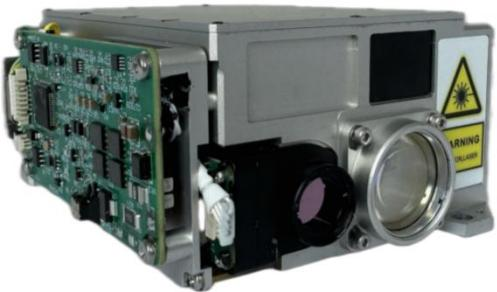
LDR80K1 1064nm Laser Rangefinder & Laser Irradiation. The ranging capability for NATO targets is  $\geq 16$  km. The ranging frequency is 1~ 20 Hz. The laser illumination distance is  $\geq 8$  km. The pulse width is  $\geq 15$  ns  $\pm 5$  ns. The beam divergence angle is  $\leq 0.30$  mrad. The weight is  $\leq 680$  g.
